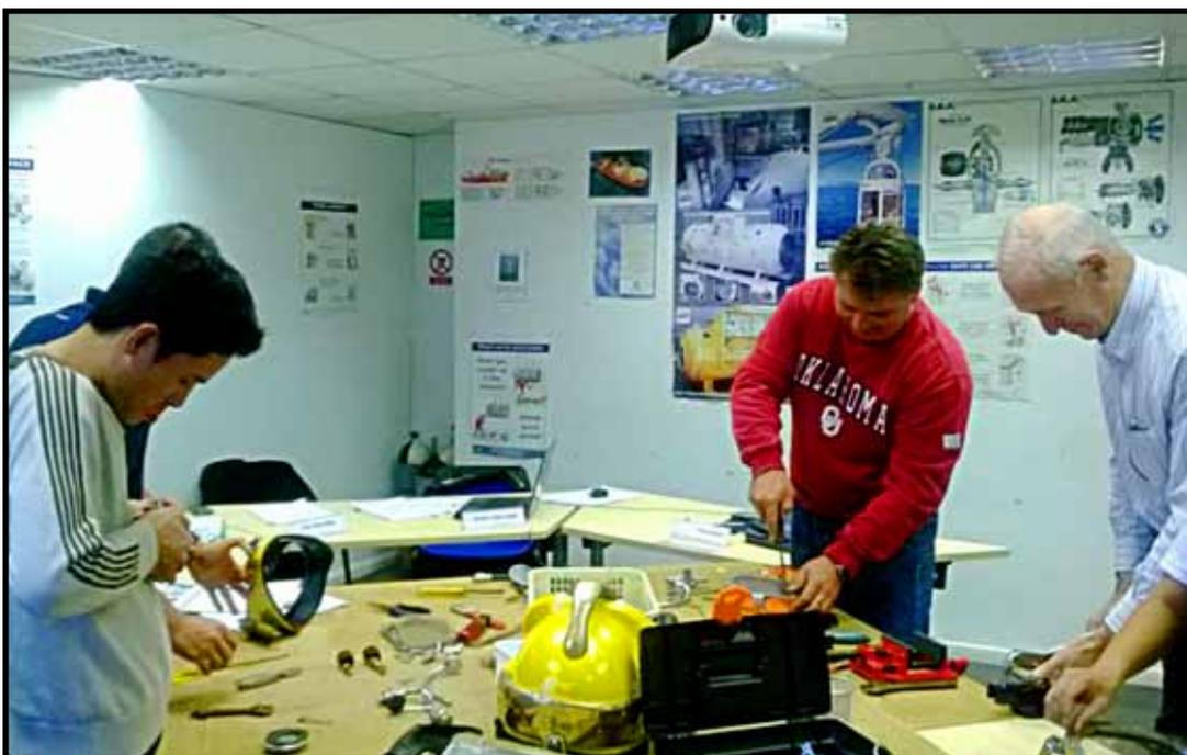
**P**ersonal Diving equipment inspection, repair & maintenance (IRM) is probably one of the most important jobs in commercial diving. The equipment is part of a divers "Life support" system and without proper care, use & maintenance, can at worst put the diver at risk, and at least, cost the employer money in breakdown time.
