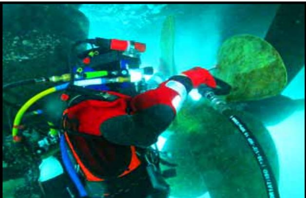
*Cleaning a propeller with Cavitchleaner*
