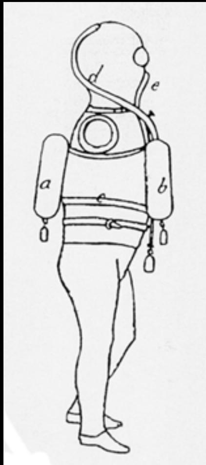
basic, as shown in the drawing. A cuirass with a metal helmet, with attached to a leather trousers and arms. This was supplied through a tube (d) from two containers 'for air' (a and b), mounted on the chest and back and 'joined by a tube' (c). The supply tube had a tap to control the air flow. In front of the mouth was an exhaust tube (e), with a valve.
